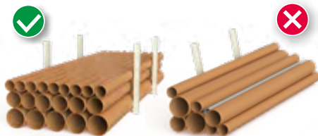
DIAGRAM 3: Correct and Incorrect way to store pipes
